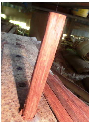
This flat piece of steel have round holes that help shape the wooden pegs that hold the wooden planks of the boat together. Picture by Satiman Jamin
