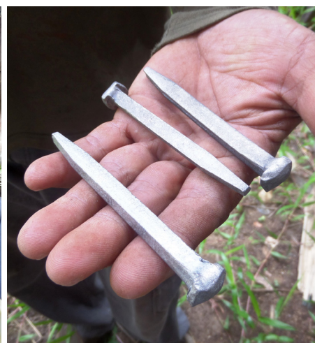
Rust-resistant steel nails are used to attach the wooden planks to the boat frame. Picture by Satiman Jamin
