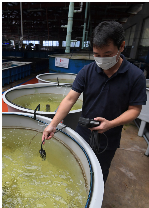
Assoc. Prof. Dr Liew examining the quality of the water in the ECO-RAS system using YSi parameter
